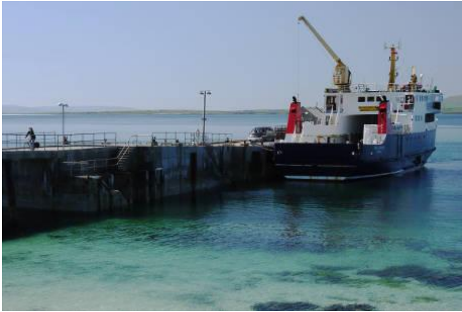
Orkney ferry MV Earl Thorfinn using its crane to lift cars onto the pier at Papa Westray.
